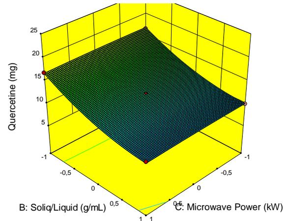
Figure 3. Three-dimensional response surface of solid-to-liquid ratio and microwave power
