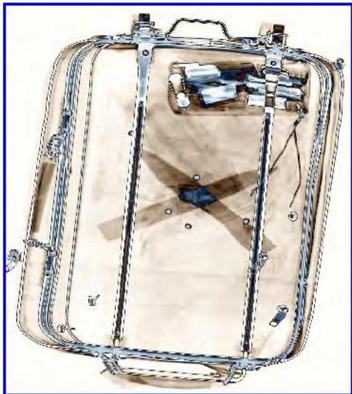
Fig. 5: (a) Original grayscale image (b) Output image obtained after applying cosine transformation clearly showing the threats (dark red and purple glass knives)
