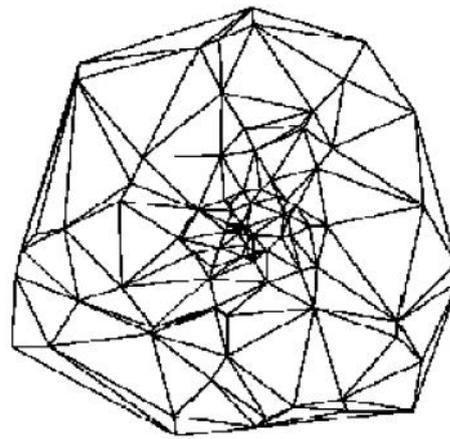
The above figure shows the Delaunay triangulation of the given set of points.
