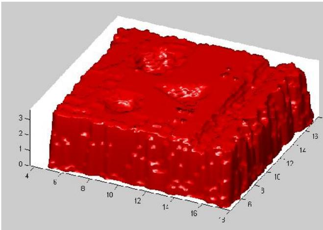
The above figure shows a 3D model of the object obtained after the filtered interpolated results were used to construct a volume data. Generation of the figure uses isosurface concept.
