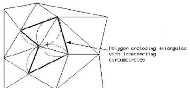
Now the vertices of the triangles and the point are so joined that the condition for Delaunay triangulation is satisfied.
